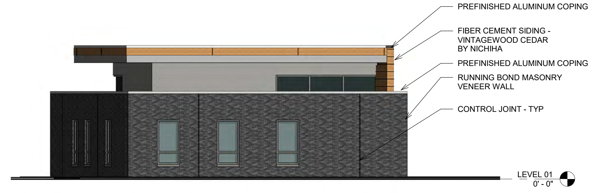
4 LEASING BUILDING - WEST ELEVATION 1/8" = 1'-0"
