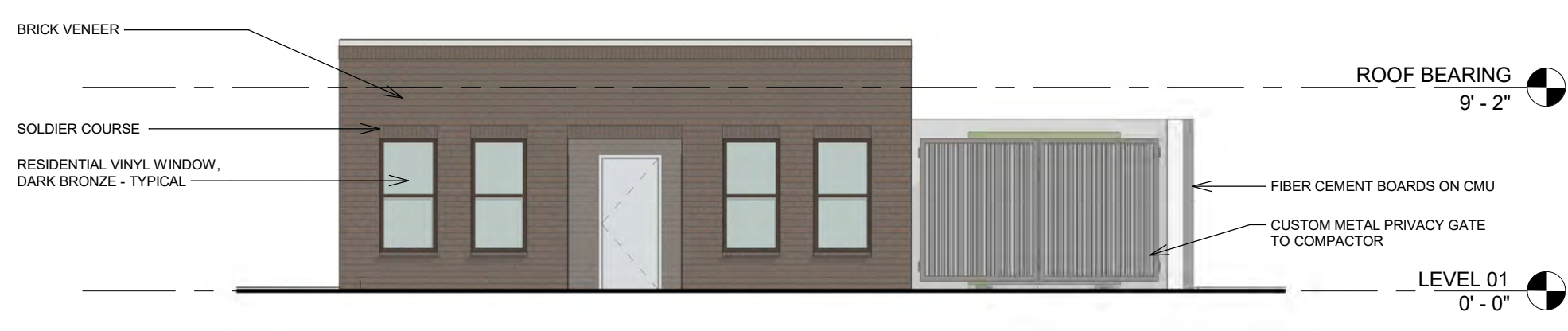
3 MAINTENANCE BUILDING - ELEVATION EAST 1/8" = 1'-0" 0' 4' 8' 16' 24'
