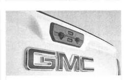
Tailgate with EZ Lift assist, power lock & release (QT5)
