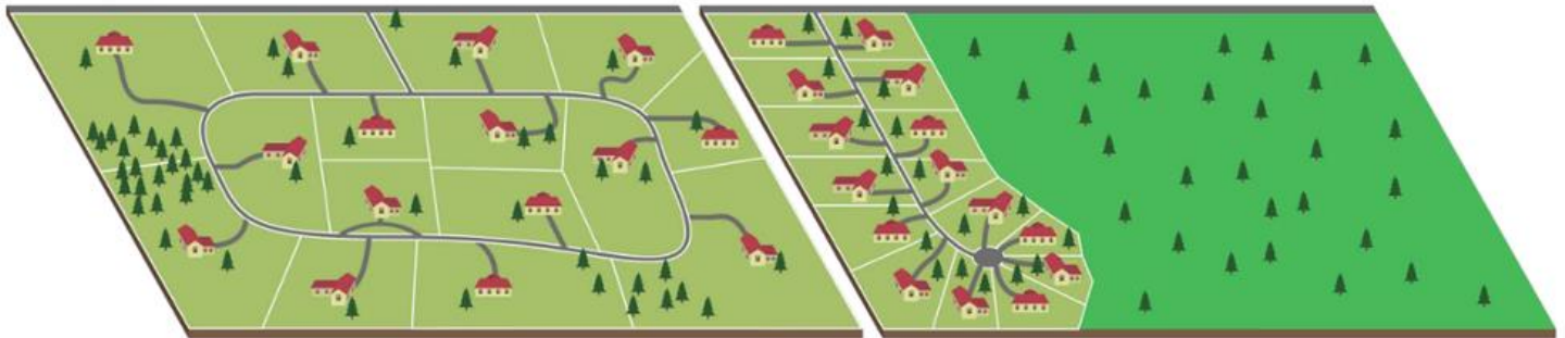
Figure 2. A conceptual example of conservation development, in which lots are grouped to a certain area, while conserving a large portion of the land's natural resources.
