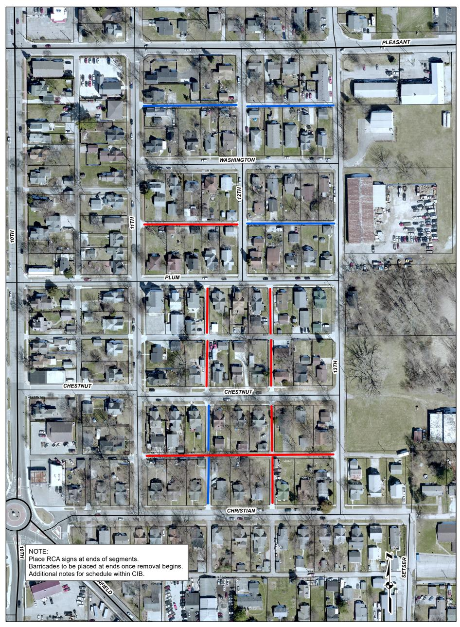
5" Mill Removal, 4" HMA Base, 1.5" HMA Surface
